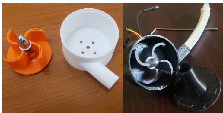
Figure 4. 3D printed pump parts and assembly with motor.
