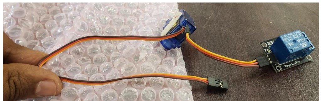
Figure 6. Physical implementation of the servo interface with relay.
